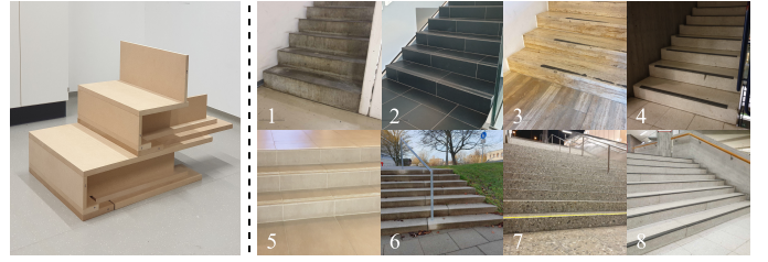
Fig. 5. The lab-constructed stairs on the left is used in training set to realize different dimension combinations. The test set on the right cover different dimensions & materials including: concrete, wood, and ceramic.
